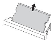
(2) Gently remove the RAM module from the slot.
