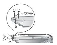
To store the stylus, push the end into (C). Push in the stylus so that the part (b) is aligned with (D).
