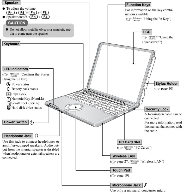
box only a monaural condenser microphone (miniature jack). Using an input source other than a monaural condenser microphone may not allow audio to be input or may damage the equipment.
