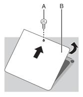
${f 2}$  Turn the computer over and remove the battery pack and the screw (A), then remove the cover (B). ( page 9)
