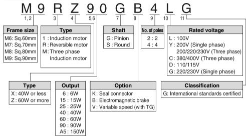
\* Induction motor and reversible motor are single phase motor.
