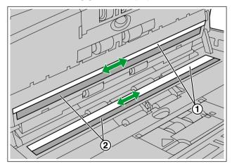
**4.** Remove dust on the double feed detectors (①) with a cotton swab.
