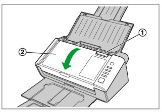
3. Clean the scanning glass area (①) and reference area (②) using a soft and dry cloth.
