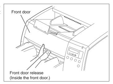
Clean the scanning section glass and sensor rollers using the accessory roller cleaning paper.
