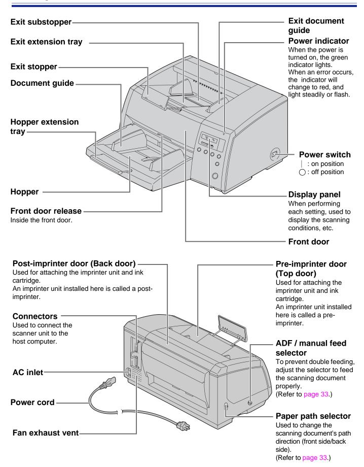
The required settings must be selected prior to scanning. Information and conditions are shown on the LCD (Liquid Crystal Display).
