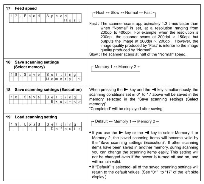
• Scanning settings 01-17 must be saved using setting "18 Save scanning settings (Execution)". Even if they are not saved, they will be applied. If the power is turned off, the next time the unit is used they will not be applied.
