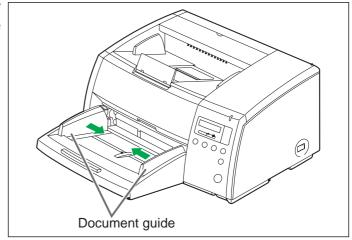
Place the documents on the hopper with the side to be scanned facing up. Then push them in the direction of the arrow until they stop.
