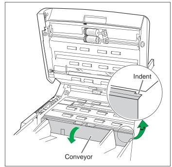
Pull the right side of the shaft in the direction of the arrow and hold it there.
