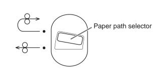
The paper path selector is located on the left side of the scanner.
