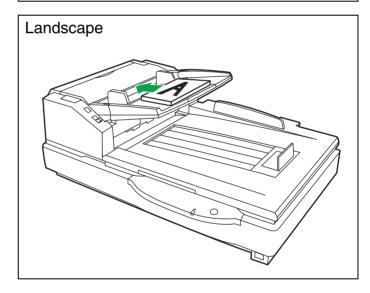
7 Adjust the document guide to the size of the document to be scanned. Adjust the exit stopper to the size of the document to be output.
