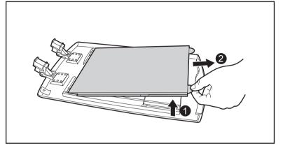
**4.** Reverse the flatbed sheet, and then place the tips of the ears of the flatbed sheet (**1**, **2**) so that they fit under the tabs of the document cover (**3**, **④**).
