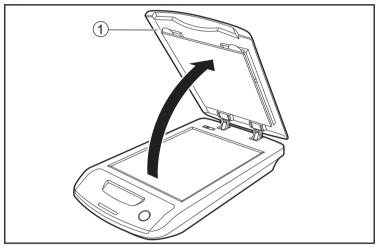
2. Place the document face down, and align the edge of the document (①) with the standard mark (②) in the upper right of the flatbed glass.
