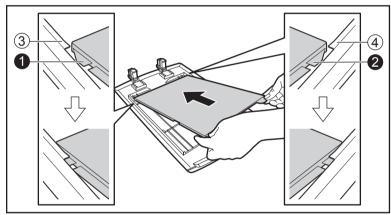
5. Push the flatbed sheet towards the rear while making sure that the ears of the flatbed sheet (①, ②) are under the tabs of the document cover (③, ④).
