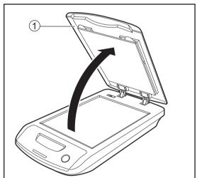
**b.** Slide the LOCK/UNLOCK selector (①) to the left to release the lock.
