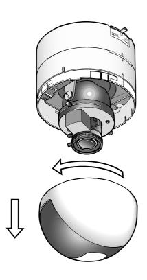
2-4. Match the slit in the camera fixing bracket with the lock line on the camera, and mount the camera onto the camera fixing bracket.
