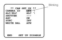
The CAM SETUP menu appears on the monitor as shown above.
