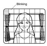
Move the cursor to the area where backlight is bright and press (S) to mask that area. The mask turns white. (When the cursor is moved on an area that has already been masked, the mask and cursor start blinking.)
