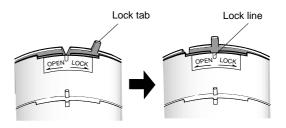
2-6. Attach the fall prevention cap on the lock tab of the camera fixing bracket as shown below to prevent the camera from falling down.
