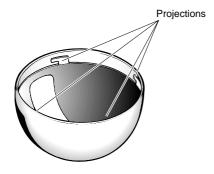
2-8. Attach the dome cover to the camera by turning this cover clockwise so that the window in the dome cover matches the camera head.
