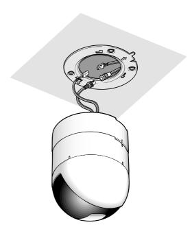
2-3. Remove the dome cover from the camera by turning it counterclockwise.
