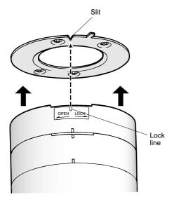
2-5. Turn the camera in the LOCK direction until the lock tab of the camera fixing bracket meets the lock line of the camera.
