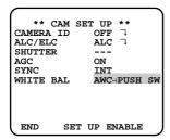
Press (S) to start the white balance setup. The words PUSH SW start blinking to indicate that the white balance is being set.
