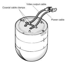
Pass the video output cable and power cable through the hole in the camera fixing bracket, and connect as described in the previous section "CONNECTION."
