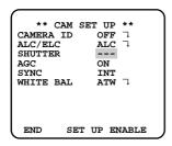
Move the cursor to the SHUTTER parameter and select the electronic shutter speed.
