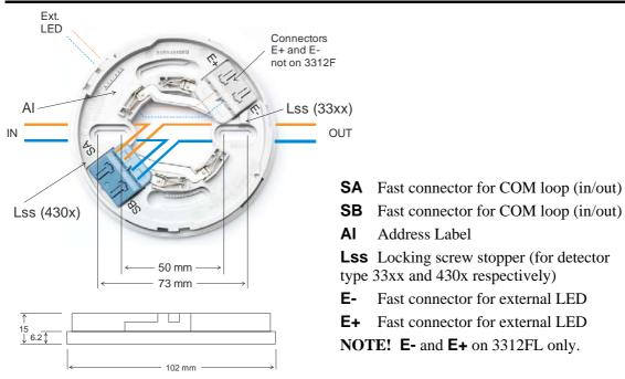
The base is prepared for mechanical locking of the detector, when a detector with a locking screw is plugged into the base. Connector wire  $\emptyset$  0.6 – 1.2 mm (approx. 0.28 – 1.13 mm<sup>2</sup>). If wire  $\emptyset$  0.6 mm is used the release button may be pushed as the wire is pressed into the connector. Analog detector types 33xx and 43xx can be plugged in the base 3312F/FL.
