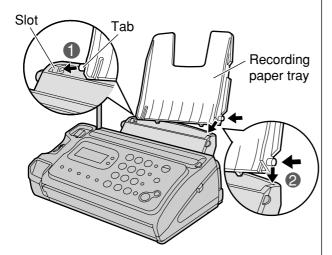
2 Insert the recording paper into the recording paper tray.Open the paper entrance cover until it locks.
