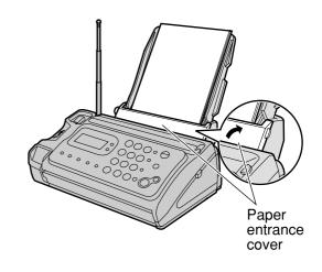
**4** Install the recording paper cover on the recording paper tray by sliding it down from the top.
