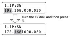
Input the IP address in four blocks of numerals. When input advances to the last block and the F2 dial is pressed, the IP address is entered.
