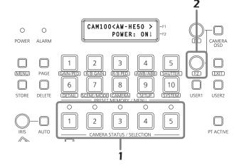
Turning on the power of a multiple number of cameras
