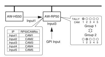
In response to inputs 1 to 5 from GPI Input, tally indicators CAM1 to CAM5 are lighted in red, and the tally ON instruction is sent to the remote cameras concerned. Only CAM1 to CAM5 serve as the GPI Input tally. This means that when a camera group other than No.1 is selected, the tally indicators will go off.
