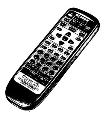
This remote control can be used to operate the receiver you purchased and some other Panasonic and Technics compact cassette decks, CD changers (and CD players), TVs, VCRs and DVD players, provided they are equipped with a remote control sensor.
