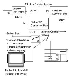
The above cable hook-up allows VCR functions, including viewing one channel while recording another, but it requires two cable TV Converter/Descrambler Boxes, one Switch Box and one 2-Way Splitter.
