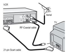
Connect all the cables as shown in the illustration, then connect the AC Mains lead (part of the package) to an AC wall outlet.
