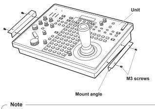
• For details on the dimensions for attaching mount angles to the unit, refer to "Appearance" (page 11).
