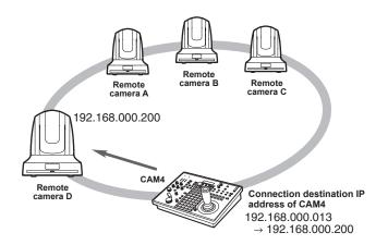
If camera numbers for which the connection type is set to other than "Serial" include a camera number for which the connection destination IP address is set to the same value as the IP address of a detected remote camera, the connection destination IP address set on the unit is not updated. The connection destination IP address is kept as is and a link is set for the corresponding camera number and remote camera.
