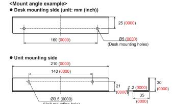
2. Attach the mount angles to the sides of the unit with four M3 screws.
