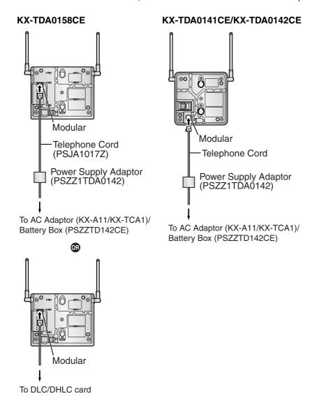
**5.** Install the CS temporarily for the site survey. Install the CS at least 2 m above the floor, keeping the antennas in the upright position.
