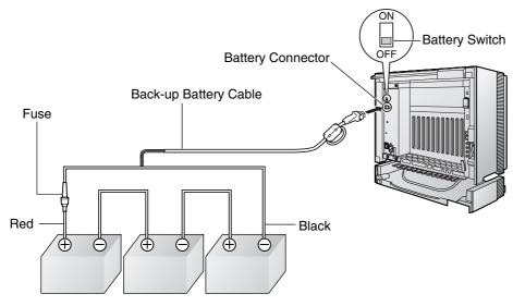
Backup Batteries (VRLA 12 V DC x 3)
