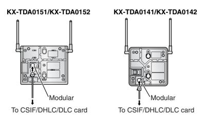
2. Pass the cable through the groove of the CS (in any direction depending on your preference).
