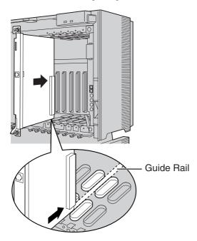
**2.** Holding the card as shown below, push the release lever in the direction of the arrow so that the card engages securely with the connector on the back board.
