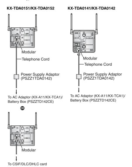
5. Install the CS temporarily for the site survey. Install the CS at least 2 m above the floor, keeping the antennas in the upright position.
