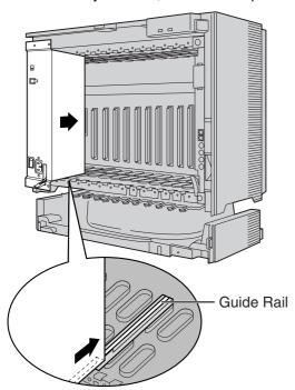
**2.** Push the release lever in the direction of the arrow, so that the PSU engages securely with the connector on the back board.
