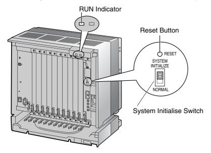
2. Plug the AC power cord into the PBX and an AC outlet, and turn on the PBX. The RUN indicator will flash.
