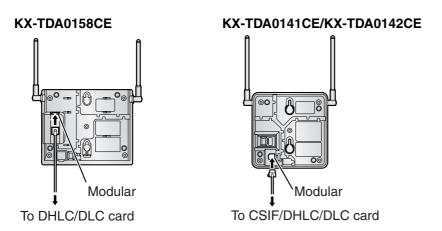
2. Pass the cable through the groove of the CS (in any direction depending on your preference).
