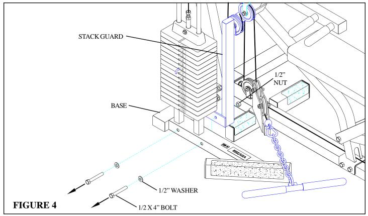
• Remove two 1/2 X 4" BOLTS, two 1/2" WASHERS, and two 1/2" LOCK NUTS from the BASE and STACK GUARD as shown in FIGURE 4. (NOTE: Discard the 1/2 X 4" BOLT.)
