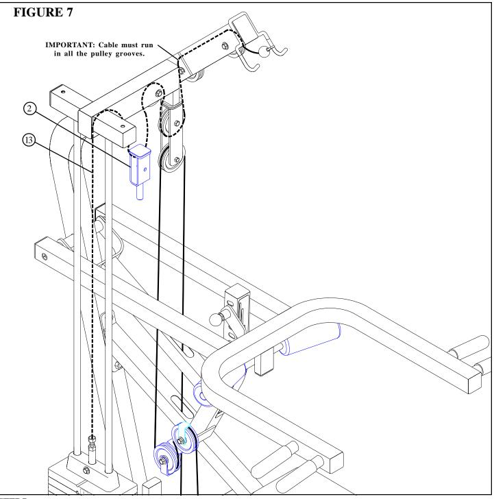
Install the NEW PRIMARY CABLE (13) using the following steps:
