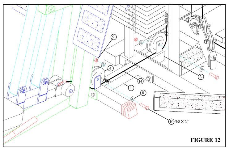
• Attach one 3-1/2" PULLEY (4) to the FRONT LEG (1) and one 3-1/2" PULLEY (4) to the BASE CONNECTION (3) using two 3/8 X 2" BOLTS (10), four 3/8" WASHERS (8) and two 3/8" LOCKNUTS (9). (Note: Make sure CABLE (14) is running under **PULLEYS.)**
