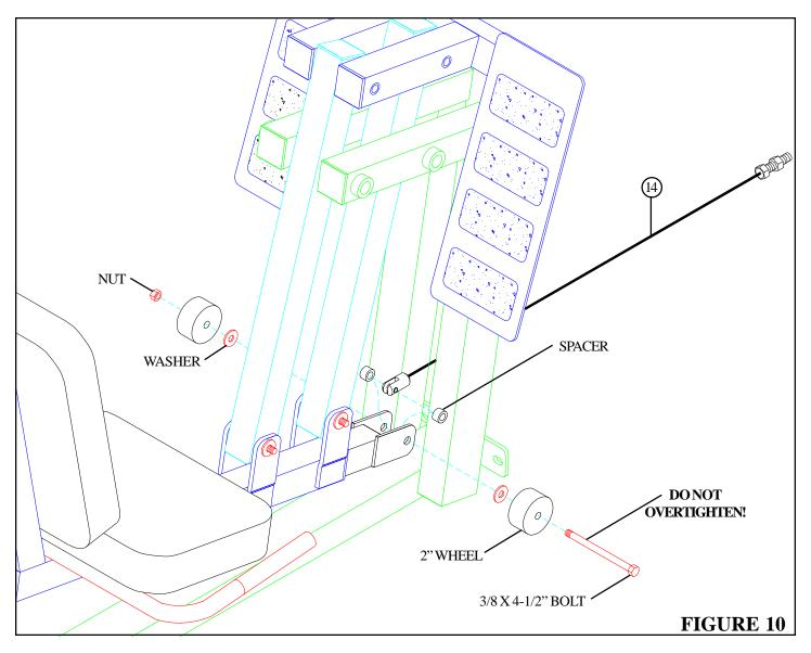
• Assemble the LEG PRESS CABLE (14) to the ADJUSTMENT TUBE on the 832 using the existing previously removed 3/8 X 4-1/2" BOLTS, SPACERS, WASHERS, 2" WHEELS AND NUT. (Note: Do not overtighten! Tighten only until nut is completely on bolt.) See FIGURE 10.
