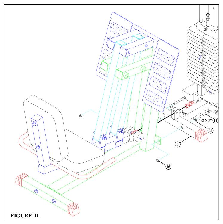
• Securely fasten the 832 LEG PRESS to the FRONT LEG (1) using two 1/2 X 3" BOLTS (11), two 1/2" WASHERS (15), and two 1/2" LOCK NUTS (16) as shown in FIGURE 11.
