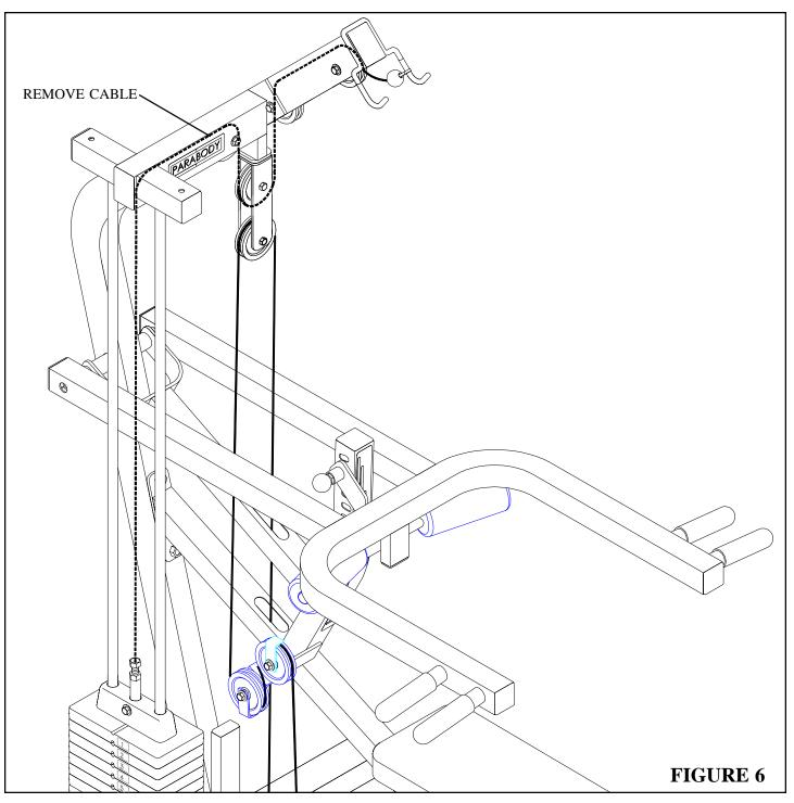
Remove the existing CABLE (part #68331) using the following steps:
