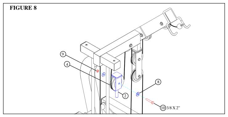
• Loop CABLE (13) around one 3-1/2" PULLEY (4) in the PULLEY BRACKET (2) and **SECURELY** assemble using one 3/8 X 2" BOLT (10), and two 3/8" WASHERS (8) and one 3/8" LOCK NUT (9) as shown in FIGURE 8.
