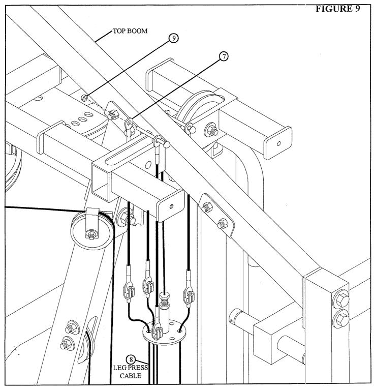
• CAREFULLY attach the TENSION CORD (7) to the corresponding small shaft on the TOP BOOM using one 1/4" CAP NUT (9) as shown in FIGURE 9.
