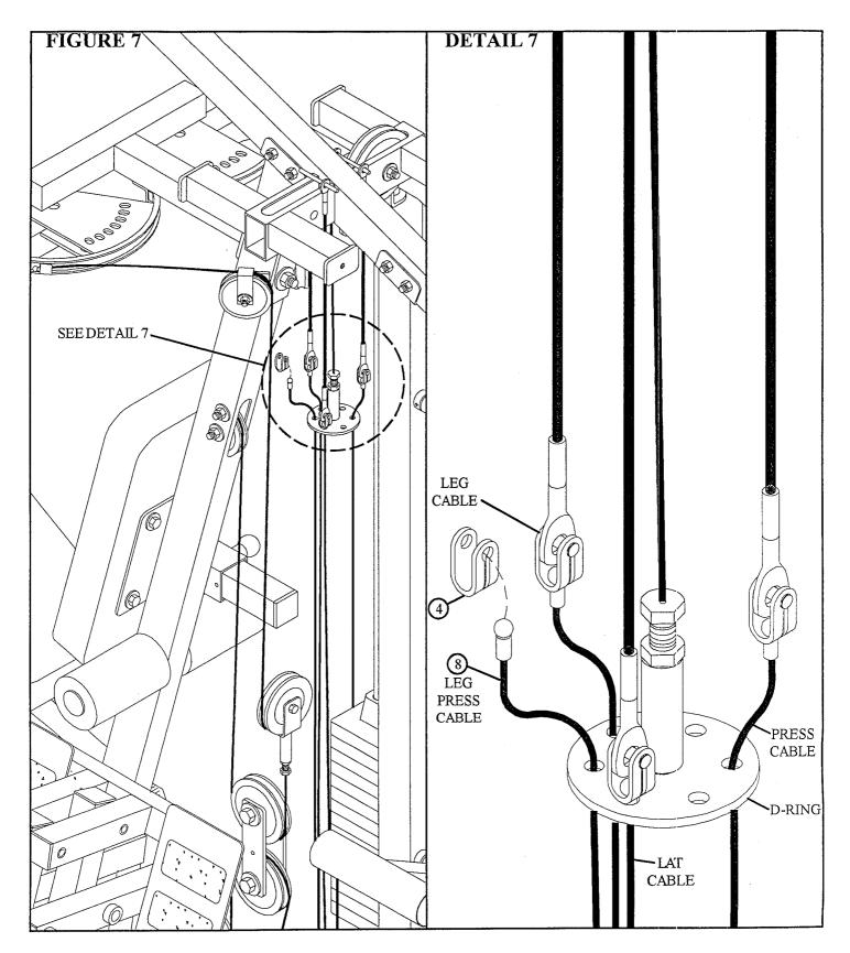
• Run the LEG PRESS CABLE (8) through the correct hole on the d-ring and attach one KEYHOLE CLEV. (4) to the end of the LEG PRESS CABLE (8). See FIGURE 7 & DETAIL 7.
