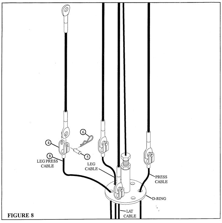
• Attach one TENSION CORD (7) to the KEYHOLE CLEVIS (4) using one CLEVIS PIN (5) and one COTTER PIN (6) as shown in FIGURE 8.
