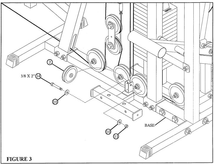
SECURELY attach one 3-1/2" PULLEY (2) to the BASE using one 3/8 X 2" BOLT (14), two 3/8" WASHERS (10), and one 3/8" LOCK NUT (11). See FIGURE 3.
