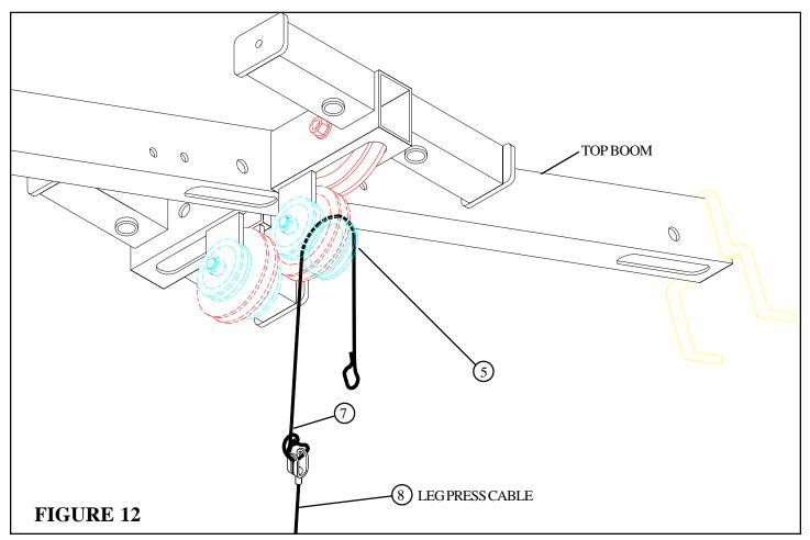
• Assemble the 72" ELASTIC CORD (7) from the LEG PRESS CABLE (8) around the 2" PULLEY (5) in the TOP BOOM as shown in FIGURE 12.
