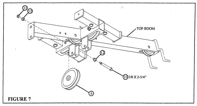
• LOOSELY assemble one 4-1/2" PULLEY (6) to the TOP BOOM using one 3/8 X 2-3/4" BOLT (13), two 3/8" FLANGE SPACERS (12), and one 3/8" LOCK NUT (11). See FIGURE 7.
