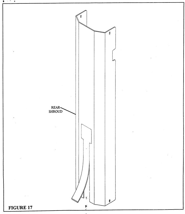
• If the 435103 LEG PRESS ADAPTER KIT is not installed the rear SHROUD opening must be removed. Apply pressure to the bottom of the SHROUD where the "V" groove is and carefuly remove the weight stack opening on the plastic SHROUD as shown in FIGURE 17.
