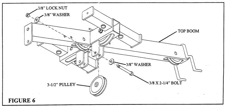
• Remove the existing 3-1/2" PULLEY, 3/8 X 2-1/4" BOLT, 3/8" WASHERS, and 3/8" LOCK NUTS from the TOP BOOM. They will be used later. See FIGURE 6..
