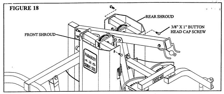
• SECURELY attach the four previously removed 3/8" X 1" BUTTON HEAD CAP SCREWS from the top of the front SHROUD & rear SHROUD. See FIGURE 18.
