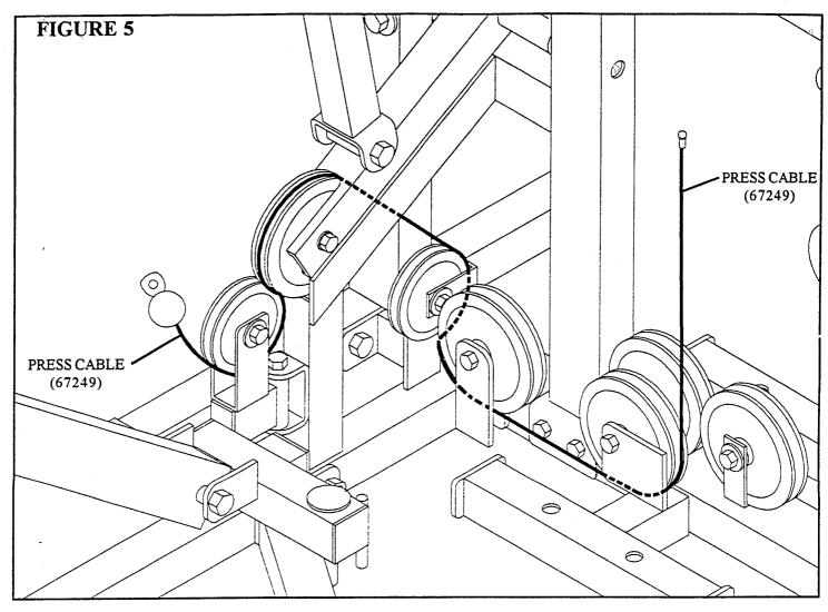
• Carefully remove and discard the PRESS CABLE as shown in FIGURE 5.
