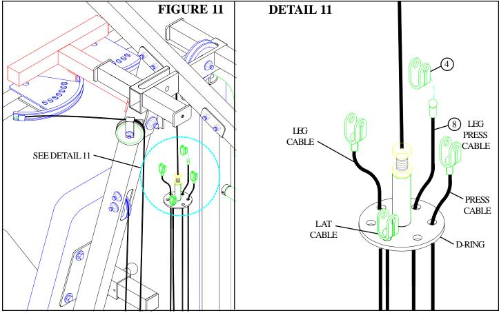
Run the LEG PRESS CABLE through the correct hole on the d-ring and attach one KEYHOLE CLEVIS to the end of the LEG PRESS CABLE. See FIGURE 11 & DETAIL 11. (NOTE: If the 663101 SECOND STACK kit is installed, evenly space the LAT & LEG EXT. CABLES on the D-RING)
