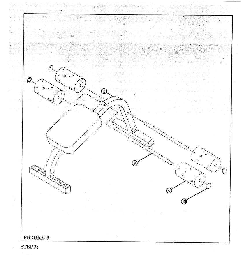
• Slide the four ROLLER PADS (8) onto two 3/4 X 16" TUBES (8) using four STARLOCK COLLARS (10) as shown in FIGURE 3.
