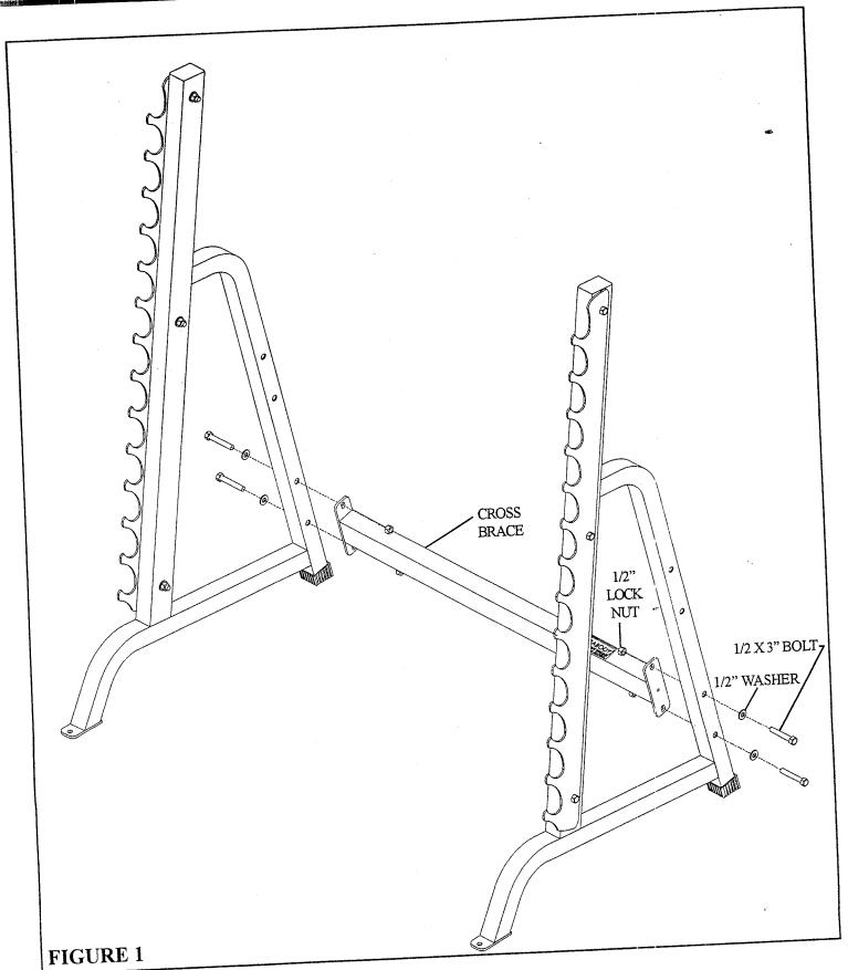
STEP 1: INSTALLATION SHOWN FOR 838101 SQUAT MACHINE. 888101 SMITH MACHINE INSTALLATION SHOWN ON PAGE 3&4.
