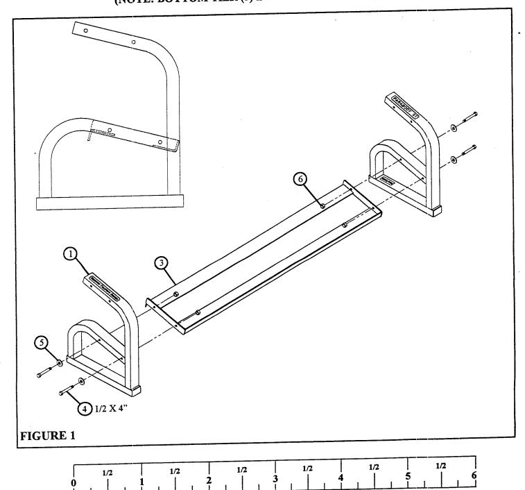
STEP 2: Loosely attach TOP TIER (2) between the UPRIGHT FRAMES (1) using four 1/2 X 4"
