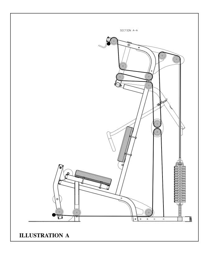
• ILLUSTRATION "A" used as cable routing reference for steps 13-16
