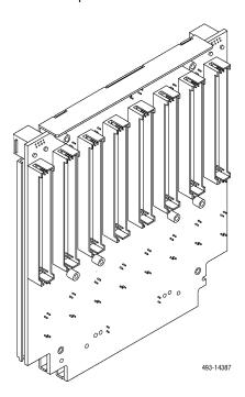
2. Attach the DTE cable (DB15) and/or port cables (DB25) to the appropriate connectors on the Auxiliary Backplane. See the COMSPHERE 3000 Series Carrier Installation Manual (3000-A2-GA31) for detailed cable and connector information. Connect the other end of the DTE cable to the customer premises equipment.
