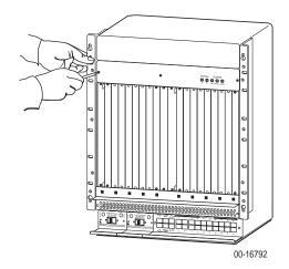
Loosen (but do not remove) the two screws on each locking bracket, and use them to slide both locking brackets toward the middle of the front panel until the ends clear the slots in the side plates.
