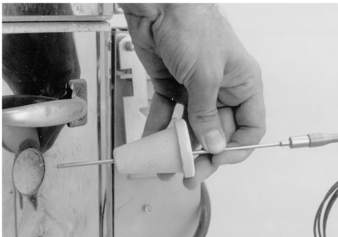
Using a drilled peephole plug to attach the thermocouple to the kiln. Make sure the thermocouple does not fall out of the kiln.
