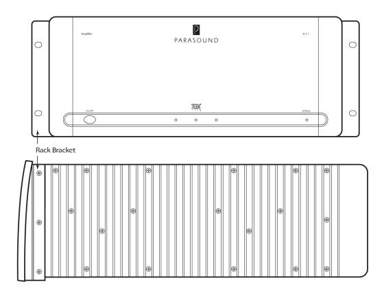
**Note:** Tighten each bolt just enough to keep the unit secure in the rack to avoid deforming the shoulder washers. Eliminating metal-to-metal contact reduces the likelihood of creating a ground loop that might introduce hum into your system.
