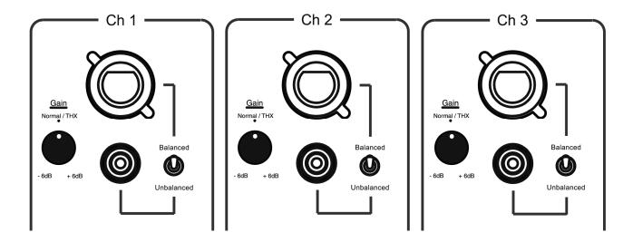
The Gain control knobs should be left at the 12 o'clock Normal/THX setting for most applications. When a Gain control knob is set to Normal the gain for that channel is 29. This is the THX Ultra2 Reference Level where 1V input = 28.28V output. (28.28V driving an  $8\Omega$  speaker equals 100 watts.) If you are unsure where to set the Gain control knobs it is best to start with them in the Normal position and only change them if needed, as described below.
