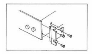
To attach the RMK-1000, first remove the three bolts at each side of the cover - closest to the front panel. Use the 6 longer bolts supplied in the rack mount kit to attach both panel extension/chassis supports.
