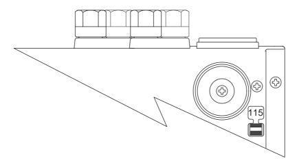
For 220-240 Vac operation. Slide the switch into the position until the section of switch labeled "230" appears through the opening in the chassis.
