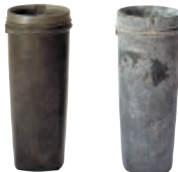
No corrosion with Alocrom treatment. Rapid corrosion of untreated aluminium.
