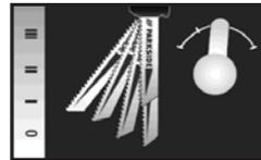
You can set the pendulum movement of the saw blade [14] using the pendulum action switch [12]. By having no pendulum action (setting "0") you can produce fine, clean cut edges. Turn off the pendulum action for thin workpieces. With the pendulum action activated (settings 1 - 3) you can cut through the workpiece at increasingly quicker rates.
