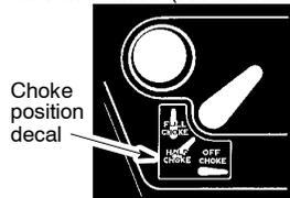
8. Pull starter rope sharply until engine runs, but no more than 6 pulls. If the engine doesn't start after 6 pulls (at the HALF CHOKE position), move the choke lever to the FULL CHOKE position and press the primer bulb 6 times. Squeeze and hold the throttle trigger and pull the starter rope 2 more times. Move the choke lever to the HALF CHOKE position and pull the starter rope until the engine runs, but no more
