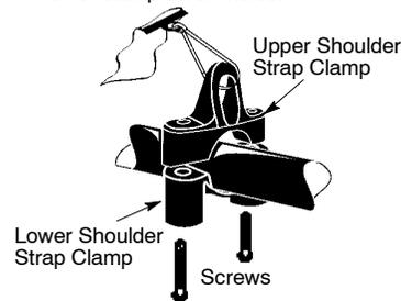
4. Insert two screws into the screw holes.
