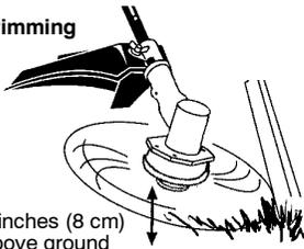
**SCALPING** - The scalping technique removes unwanted vegetation down to the ground. Hold the bottom of the trimmer head about 3 in. (8 cm) above the ground and at an angle. Allow the tip of the line to strike the ground around trees, posts, monuments, etc. This technique increases line wear.
