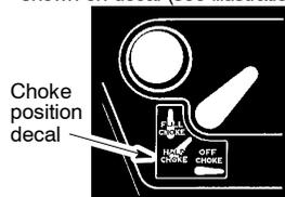
8. Pull starter rope sharply until engine runs, but no more than 6 pulls. If the engine doesn't start after 6 pulls (at the HALF CHOKE position), move the choke lever to the FULL CHOKE position and press the primer bulb 6 times. Squeeze and hold the throttle trigger and pull the starter rope 2 more times. Move the choke lever to the HALF CHOKE position and pull the starter rope until the engine runs, but no more
