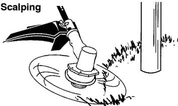
**MOWING** - Your trimmer is ideal for mowing in places conventional lawn mowers cannot reach. In the mowing position, keep the line parallel to the ground. Avoid pressing the head into the ground as this can scalp the ground and damage the tool.
