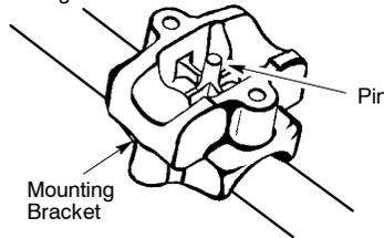
3. Position the bracket cover over the handlebar. Again make sure the handlebar is at the end of the arrow.
