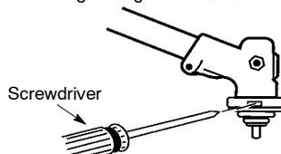
9. Tighten blade nut firmly with a wrench while holding screwdriver in position.
