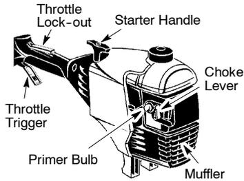
**NOTE:** The throttle lock-out is designed to prevent unintentional use of the throttle trigger. The lock-out must be pressed with the palm of your hand as you grip the throttle handle before the trigger can be used.
