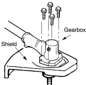
2. Insert and thread the 4 mounting screws through the holes of the gearbox and the metal shield. Tighten evenly and securely with the hex wrench provided.
