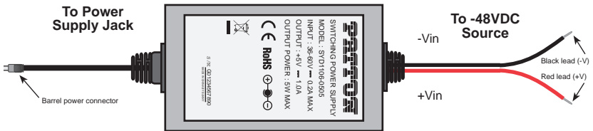
Figure 10. Connecting DC Power to the 48V-PSM DC Power Supply
