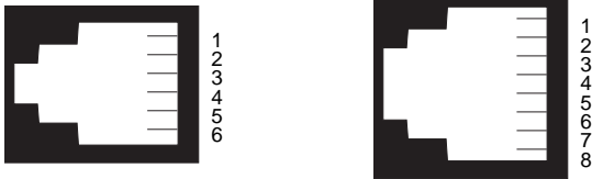
AT&T standard modular pin assignments
