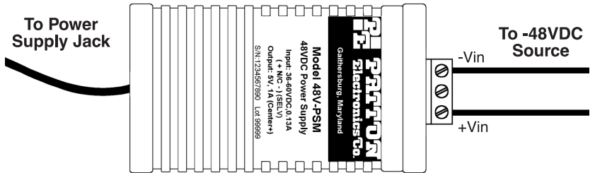
Figure 6. Connecting DC power to the 48V-PSM DC power supply
