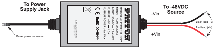
Figure 5. Connecting DC Power to the 2707 DC Power Supply
