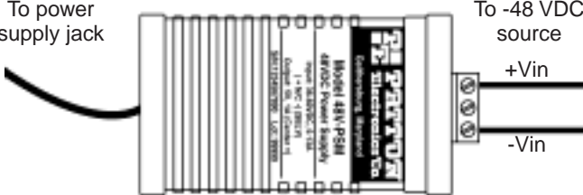
Figure 10. Connecting DC power to the 2707/I DC power supply
