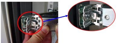
4. Simultaneously press down the right end of the locking mechanism and push the left end gently forwards to lock it into the hole at the end of the rack rail. The installation of the cable arm is completed at this point. Users may tidy the server cables up and tie-wrap them to the cable arm.
