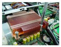
Note: The heat sink has to be installed to prevent the CPU from overheating.
