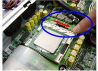
5. Place the heat sink on top of CPU1 and secure the screws on both sides.
