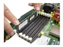
2. For optimal system performance, at least two memory modules must be installed.
