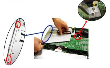
6. Push the riser card bracket carefully down with even force on both sides.
