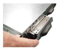
6. Screw the HDD set securely back to the system.
