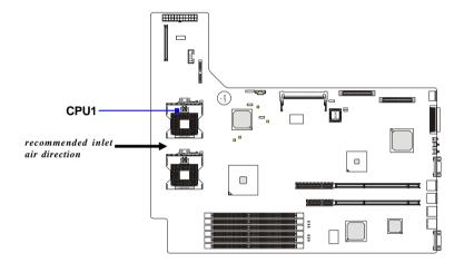
To install DUAL CPUs on the board, you must use the same type of CPUs running at the same FSB frequency.
