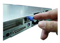
2. Press the release buttons and slide the rear chassis cover backwards to remove it from the chassis.
