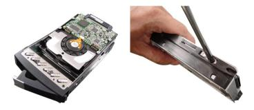
4. Insert the HDD set into the bay and press the lever back in place.
