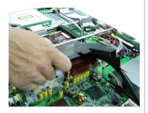
2. Locate the first CPU socket and raise the lever up to its full extent.
