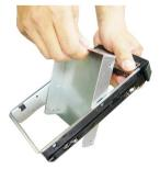
4. At the sides of the HDD are four screw holes, two on each side. Users will find on the HDD rack four identical screw holes as on the HDD. Place the HDD into the rack and align the screw holes on the HDD with the ones on the rack. Secure the HDD with four screws supplied by the HDD vendor.
