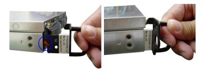
2. Push it in until it fits firmly. Screw to secure the chassis ear.
