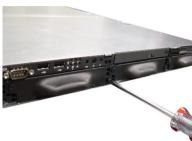
2. As the system mainboard supports two Serial ATA HDDs, only the HDD trays on the right & left sides can be used.
