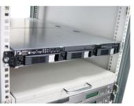
3. Screw the system firmly to the rack.
