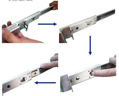
5. On each side of the chassis are three hooks to lock the chassis rail. First align the chassis hooks with the holes on the rail. Secure the rail to the chassis and push the rail backwards until it gets locked by the chassis hooks.
