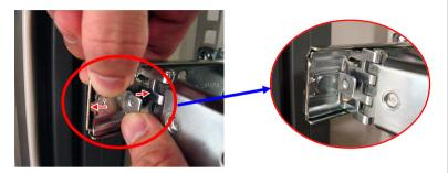
5. A screw-knob is designed for users to adjust the angles (up or down) of the cable arm. Use a screwdriver to turn the screw-knob clockwise or counterclockwise and the cable arm will go up or down.
