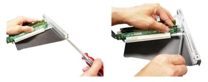
3. Insert the expansion card into an appropriate PCI slot on the riser card and secure the screw with a screwdriver.
