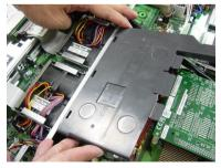
Note: To ensure proper cooling, make sure the heatsinks & the fan duct are properly installed.
