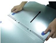
3. Press the release buttons and slide the front chassis cover forwards to remove it from the chassis.
