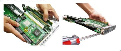
4. Install the second PCI expansion card if necessary.
