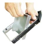
3. At the sides of the HDD are four screw holes, two on each side. Users will find on the HDD rack four identical screw holes as on the HDD. Place the HDD into the rack and align the screw holes on the HDD with the ones on the rack. Secure the HDD with four screws supplied by the HDD vendor.
