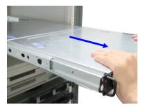
2. The system will be locked halfway while being pulled out. Simultaneously press down the locking tabs on both sides of the chassis and pull the system forwards. The system should slide easily off the rack.
