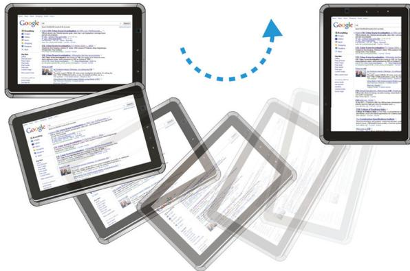
This function can be enabled/ disabled by G-sensor Lock.
