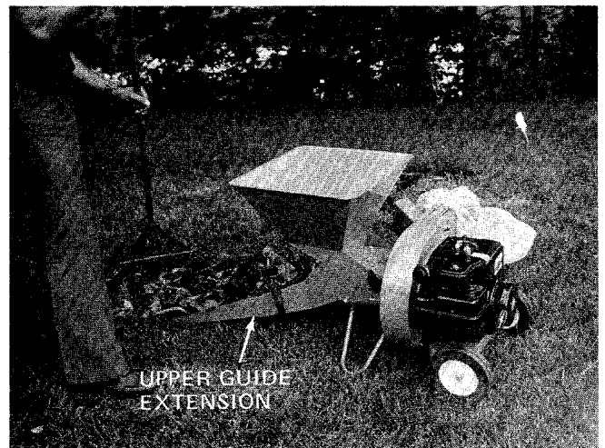
FIGURE 11. RAKING LEAVES AND TWIGS INTO UPPER GUIDE EXTENSION
