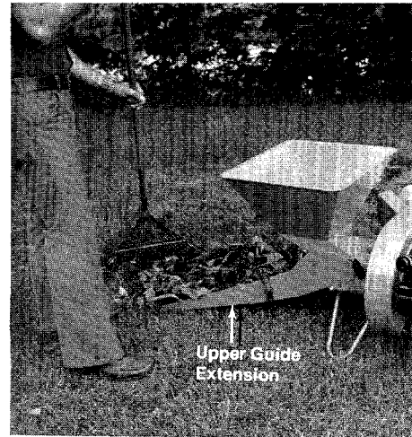
FIGURE 9. RAKING LEAVES AND TWIGS INTO UPPER GUIDE EXTENSION
