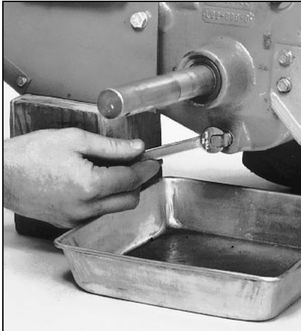
Figure 5-3: Remove drain plug to drain transmission gear oil (also remove oil fill plug and oil level check plug).
