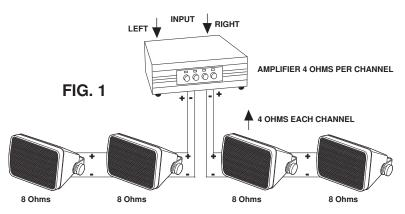
Be sure to use a good quality, unshielded twisted pair speaker cable to connect the amplifier to the speaker(s) (#14AWG for runs <80', #12AWG for runs >80').
