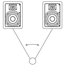
For best stereo imaging, we recommend that the units be placed so that the tweeters are as close as possible to the ear level of a seated listener. As this is not always possible in keeping with aesthetic design of a particular room, MODEL 520W, 620W, and 820W In-Wall Loudspeakers were designed with a pivoting tweeter which rotates to allow you to "aim" the high frequencies
