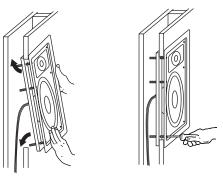
STEP 5 After speaker panel is seared tightly, test for sound.
