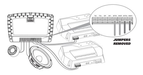
Note: It is important to make sure the gain of each amplifier is matched. Final gain level adjustments should be made using the crossover settings.
