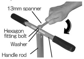
Mount the assembled rod handle on the rear of the main body. Tighten the two fitting screws using the 6mm wrench.
