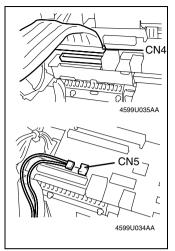
If the hard disk drive kit is installed, disconnect the connectors from CN4 and CN5 on the CLAN circuit board.
