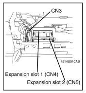
With the Di3510f, Di3010f, Di2510f and Di2010f, disconnect the Ni-MH battery cable from CN3 on the MFB3 circuit board (in order to prevent damage to the memory IC).
