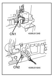
2. Disconnect the connectors from CN1 and CN2 on the power supply circuit board.
