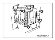
Remove the mechanical circuit board cover (5 screws).
