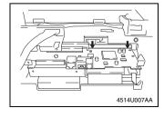
\* When installing the CLAN circuit board, press down at the two points indicated by arrows, and then firmly insert the connectors. (Do not touch any soldered areas.)
