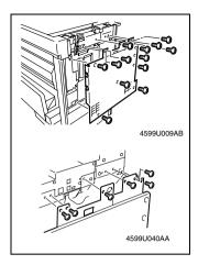
5. Remove the back panel (13 screws). (To remove the panel, slightly lift it up.)
