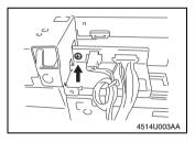
7. Remove the connector bracket (1 screw).
