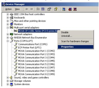
3. Basic information about the board is displayed on the **General** page. Click the **Ports Configuration** tab to configure the board's serial ports.
