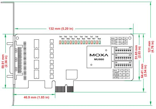
NOTE: Use JP1/2/3/4/5/6/7/8 to activate the Termination Resistors for ports 1/2/3/4/5/6/7/8. Termination Resistor is NOT active Open Short
