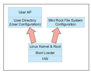
The EM-1240-LX uses ROMFS for the Linux kernel image, Root File System, and Protected configuration, and uses JFFS2 for the User Directory.
