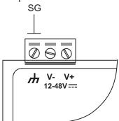
**SG**: The *Shielded Ground* (sometimes called Protected Ground) contact is the left most contact of the 3-pin power terminal block connector when viewed from the angle shown here. Connect the SG wire to an appropriate grounded metal surface.
