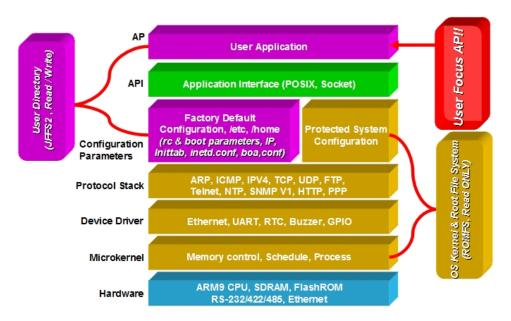
The EM-1240-LX's Flash ROM has more than one smaller partition, which contain the Boot Loader, Linux Kernel & Root (/) File System Image, and User Directory partitions.
